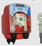
Peristaltic pump controlled by conductivity with inductive probe Range 100...30.000  $\mu$ S (30 mS) Over feed alarm, settable from 0 to 999 seconds.
