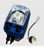
Peristaltic pump controlled by conductivity with electrode's probe Range 240...20.000  $\mu$ S (20 mS) Over feed alarm, settable from 0 to 999 seconds. Pump stops if the probe is dry
