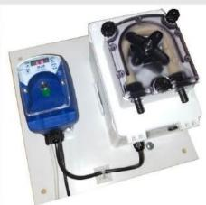
Peristaltic pump controlled by conductivity with electrode's probe Range 240...20.000  $\mu$ S (20 mS) Over feed alarm, settable from 0 to 999 seconds.
